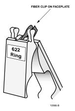
Figure 701-8. Faceplate Fiber Clip on Optical Card (622 shown)
